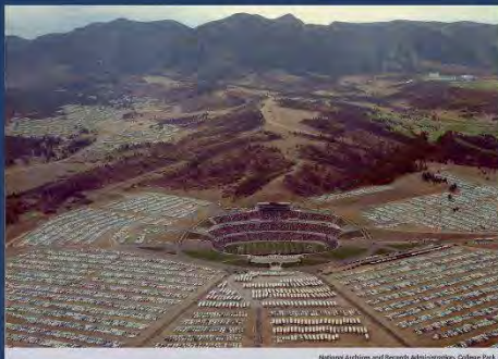
From the upper row of seating, along the foothills of the Douglas Mesa to the parking lots at the valley below, the terrain gently slopes with an approximate 100 ft elevation change. The parking field is located approximately 25 ft below the elevation of the north and south entrances. The elliptical bowl stadium design provides optimal views to the activity on the field from every seat in the stadium. (1964)
