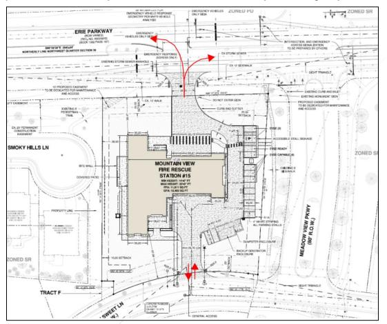
Due to close the proximity with the adjacent intersection of Meadow View Parkway and Erie Parkway, Town staff determined it would be necessary to also install a new traffic signal at the intersection to ensure safety for pedestrians and regular traffic flow, while new emergency signals will provide a dedicated control mechanism for emergency vehicles. A new break in the median will allow the left turn onto westbound Erie Parkway for exiting emergency vehicles.
