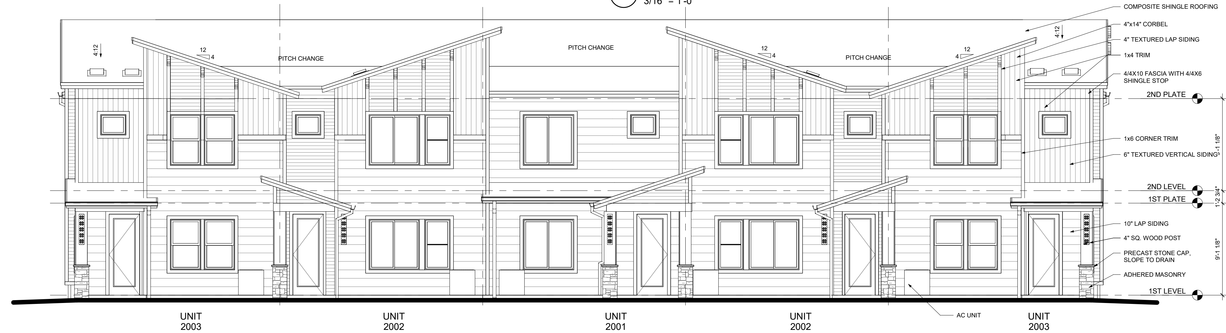
1 5-PLEX - FRONT ELEVATION - MID-CENTURY MODERN 3/16" = 1'-0"
