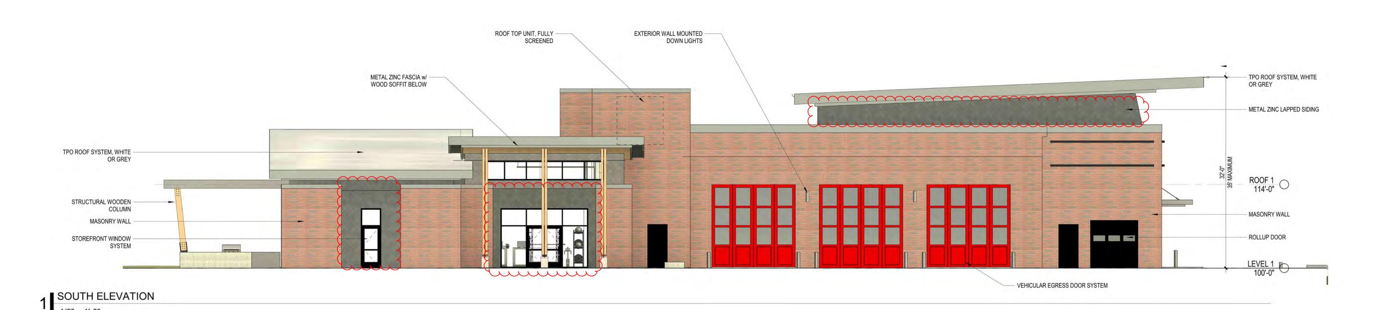
ROOF TOP UNIT, FULLY -SCREENED TPO ROOF SYSTEM, WHITE OR GREY METAL ZINC FASCIA w/ -WOOD SOFFIT BELOW STRUCTURAL WOODEN METAL ZINC LAPPED SIDING COLUMN - MASONRY WALL MASONRY WALL STOREFRONT WINDOW SYSTEM STOREFRONT WINDOW SYSTEM FENCE / SCREEN WALL
