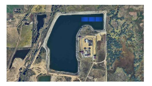
The floating solar PV system will be placed on the pond close to the Solids Building and Re-Use Pump Station – placing the system close to the buildings will help reduce cost and losses.
