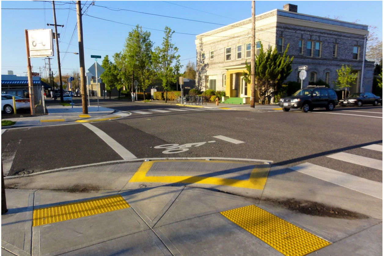
Figure 9: Recessed Stop Bar (Source: NACTO)
