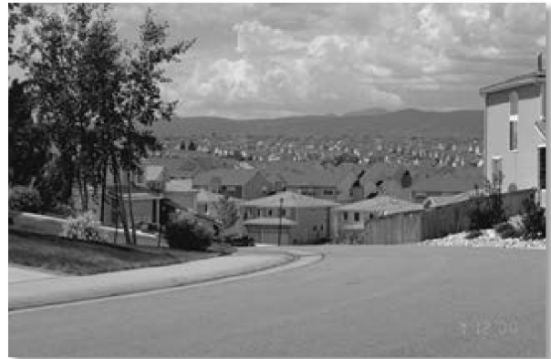
Photograph 6-2. Urbanization (impervious area) increases runoff volumes, peak discharges, frequency of runoff, and receiving stream degradation.
