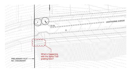
Grading for the Spine Trail appears to be incomplete on Sheet L1.8.
