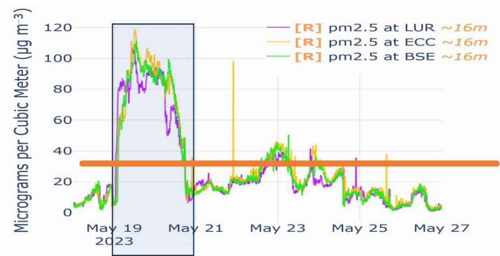
Figure 3. Time series graph of PM 2.5 (1-minute data) from 18-27 May 2023 for Erie (yellow), Longmont (pink), and Broomfield (green). The Canadian Wildfire smoke event is shown with the shaded box. The 24-hour average NAAQS is shown with the orange horizontal line.
