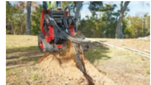
HIGH-TORQUE TRENCHER HEAD Guarantees performance in difficult soil conditions. 24", 36" and 48"* booms available. Chain speed: 120 rpm at 11 gpm. Torque: 675 ft/lbs at 3000 psi *Optional spoils auger recommended for 4' boom
