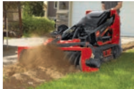
TRENCH FILLER Two sets of opposing augers direct spoils into the hole. Standard float mechanism allows for up to 5" of ground following floatation. Skids evenly disperses weight and slide easily over turf, minimizing damage.
